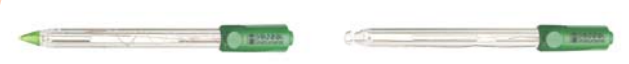
HI10530 Triple ceramic, double junction, glass body, refillable pH electrode with conical tip and temperature sensor Recommended for fats, creams, soil and low conductivity samples
