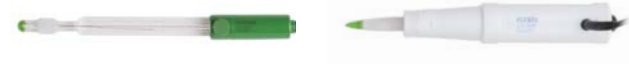
HI10480 PTFE reference, double junction, Clogging Prevention System (CPS), glass body pH electrode with temperature sensor Recommended for wine analysis and solutions with a high concentration of suspended solids
