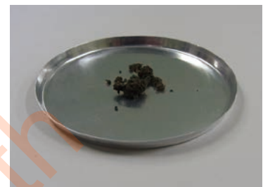
(After measurement) It whitened slightly, and the volume decreased from the drying.
