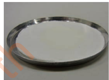
(After measurement) The moisture has evaporated from the milk, and the remaining fats have yellowed slightly.
