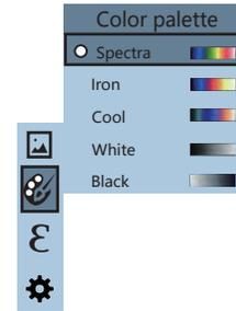
As shown in the figure, press “⏏/MENU” key to enter the main menu and select “🎨” (color palette) option and press “▶” key to enter the color palette list. Press “▲” and “▼” keys in navigation to select the color palette. Then press “SELECT/ENTER” key to select the color palette. Press “◀” to return. Press “⏏/MENU” key to exit from the menu.
