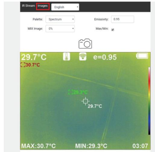
Click "Image" in the mobile device to enter the image view, press the image to download the image, long press the image to save to the mobile device, click "Infrared Video Stream" to return to the video stream webpage, as shown below.
