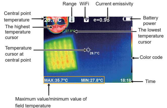
Range: The range of temperature measurements.
