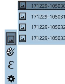
As shown in the figure, Then press “▶️” key to enter image list. Press “▲” or “▼” key in navigation to select the image. Then press “SELECT/ENTER” key to view image. When viewing the images, press “◀️” key to view the precious image, Press “▶️” to view the next image. Press “SELECT/ENTER” key to return. Press “⏻/MENU” key to exit from the menu.
