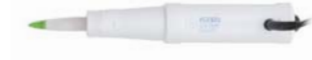
FC2320 Open viscolene reference electrolyte, double junction, PVDF body pH electrode with conical tip and temperature sensor Recommended for meat applications with use of optional FC098 20 mm (0.8") or FC099 35 mm (1.4") stainless steel blade
