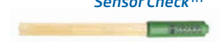
HI12301 Single ceramic, double junction, gel filled, PEI body, pH electrode with temperature sensor and matching pin Recommended for field applications
