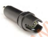
These meters also feature the HI73127 replaceable electrode with a stainless steel round connector and extendable cloth junction. This cartridge design has no pins to line up or that can break.
