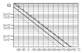
Since the resistance of the pH electrode is in the range of 50-200 M $\Omega$ , the current across the membrane is in the pico Ampere range. Large currents can disturb the calibration of the electrode for many hours.
